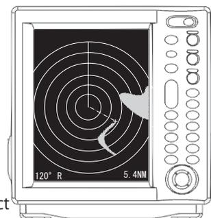
**Anti-Sea Clutter:** (STC)- A control which reduces the sensitivity of the receiver at a short range. The "anti-sea clutter" control reduces the echoes of sea clutter, which is strongest near the origin of the radar signal. (similar to surface clarity in sonar).
