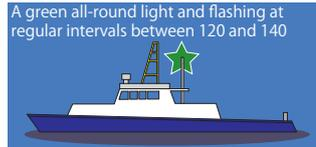
③ Vessel engaged in emergency work
